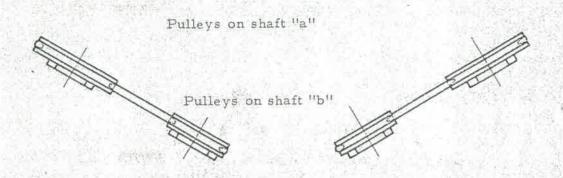
For gightening or releasing the V-belts turn screw (39) page 15 either to the right or to the left.
